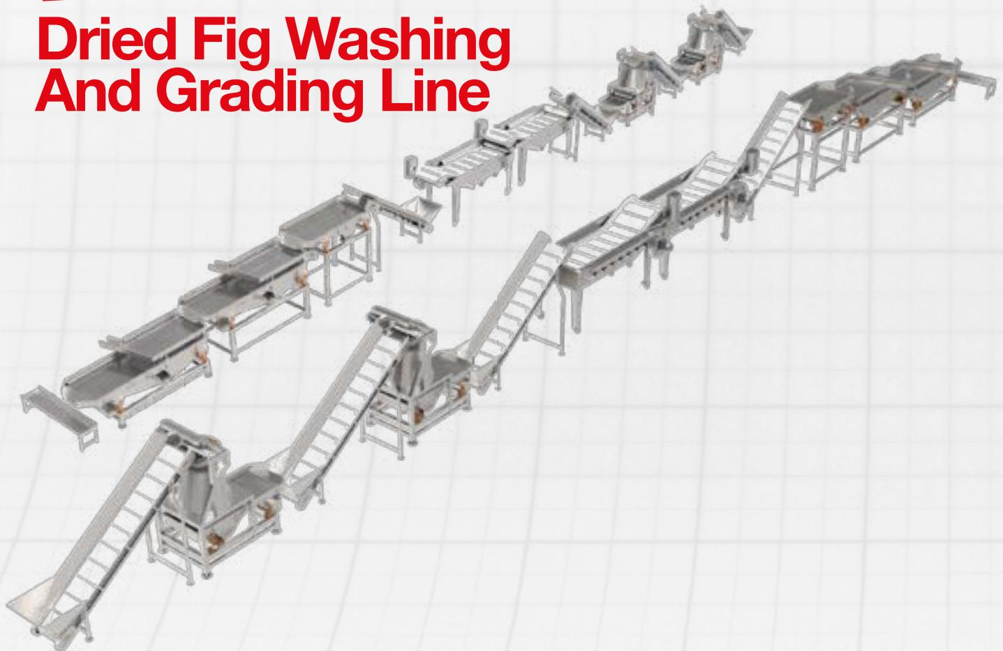
The ability of processing products from minimum 1 ton to maximum 10 tons per hour.
