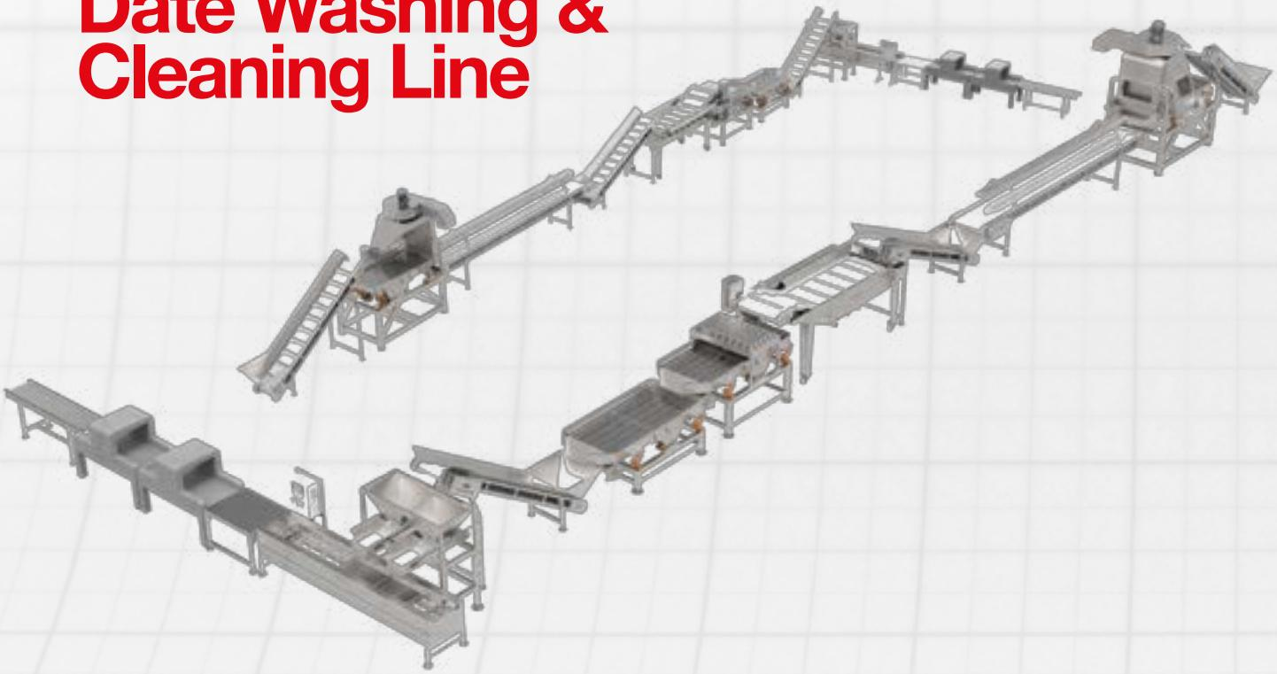
The ability of processing products from minimum 1 ton to maximum 10 tons per hour
